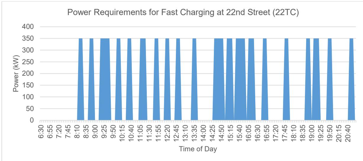
Similar to KTC, the analysis shows that one fast-charging unit of 350 kW is required, based on the modeling to successfully operate the service. However, BFT should consider installing an additional back-up charger as well.
