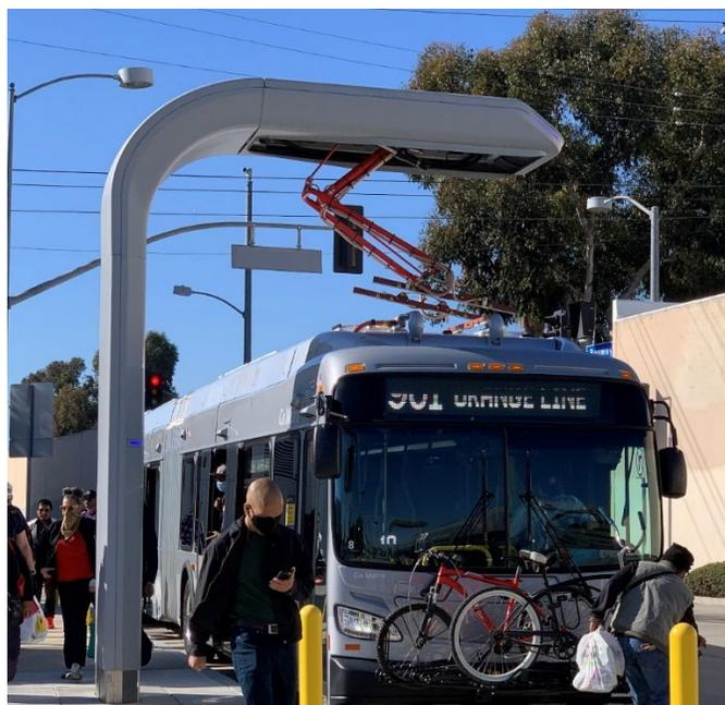
The methodology used for on-route modeling considers existing blocks and identifies currently scheduled layovers. Layovers that can be utilized for on-route charging generally include layovers that are five minutes or longer. This time window provides enough time for the bus to align with the charger, receive a significant charge, and depart the charger within the allocated time.
