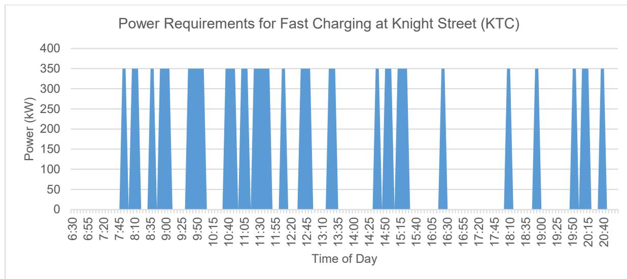
The analysis shows that one fast-charging unit of 350 kW is needed to actively recharge vehicles throughout the day; nevertheless, operationally, one spare charger should be installed at the KTC for redundancy in case of equipment failures, and/or if buses fall behind schedule affecting the availability of the primary charger.
