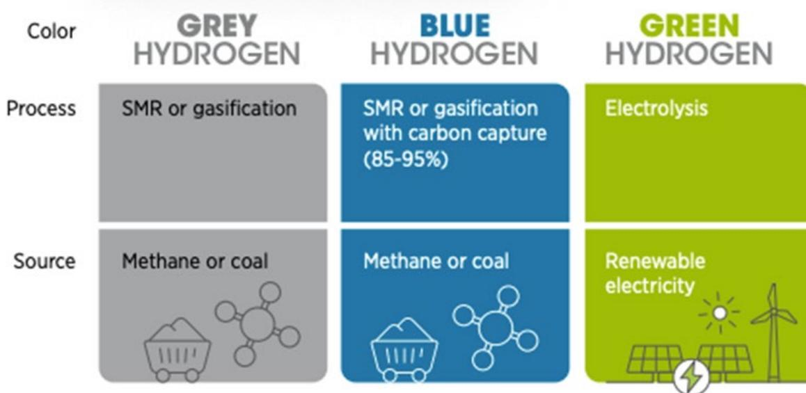
**Figure 41: Hydrogen classification based on carbon intensity**
