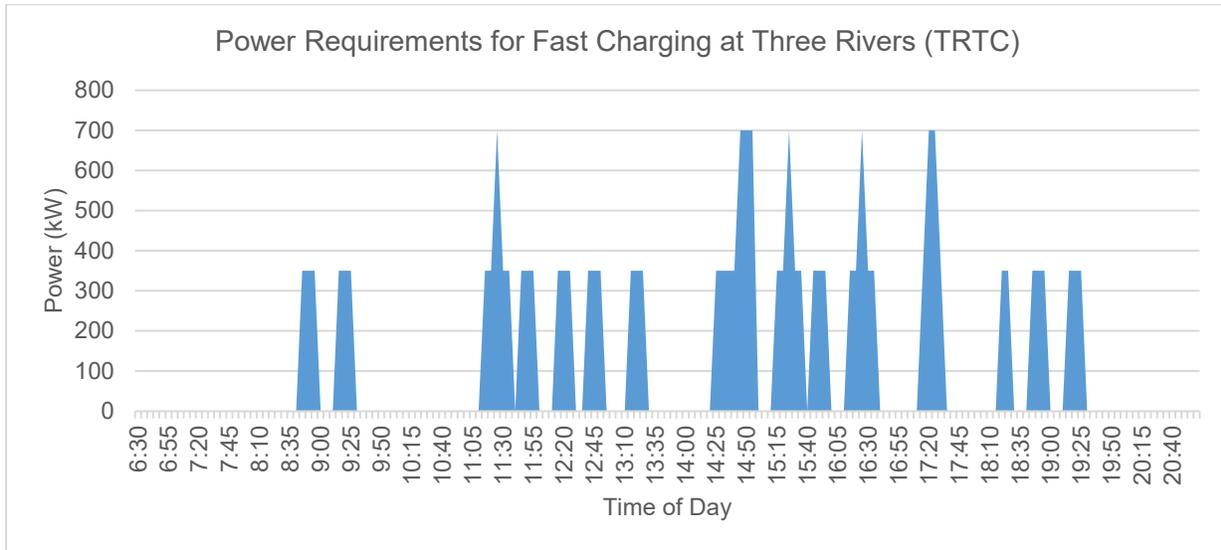
Table 11 presents a summary of the charging equipment requirements at each transit center, as well as the minimum power demand that is expected and the recommended installed capacity that is based on the capacity of the installed equipment. Two fast charging units, each at 350 kW, are recommended for KTC and 22TC and three charging units are recommended for TRTC.
