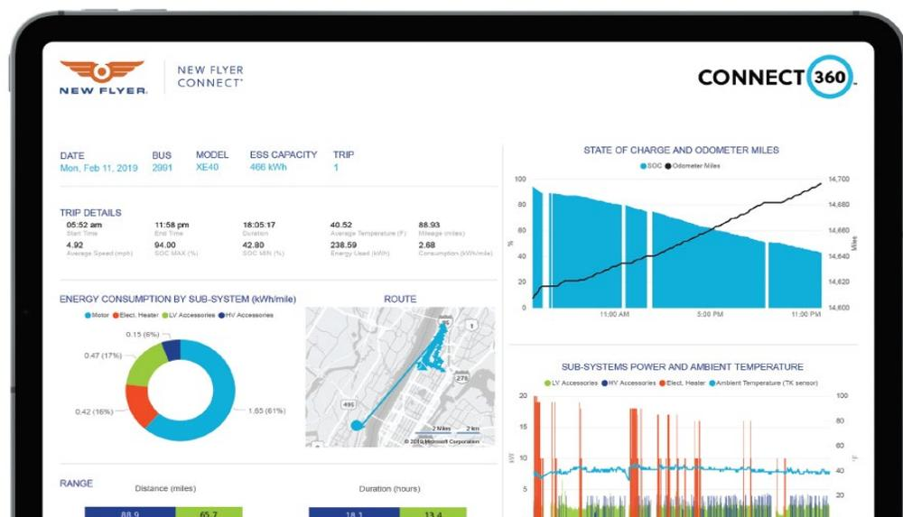
At a minimum, the fleet tracking software should track a vehicle’s SOC, energy consumption, distance traveled, hours online, etc. Tracking these KPIs can help compare a vehicle’s performance on different routes, under different ambient conditions, and even by different operators.
