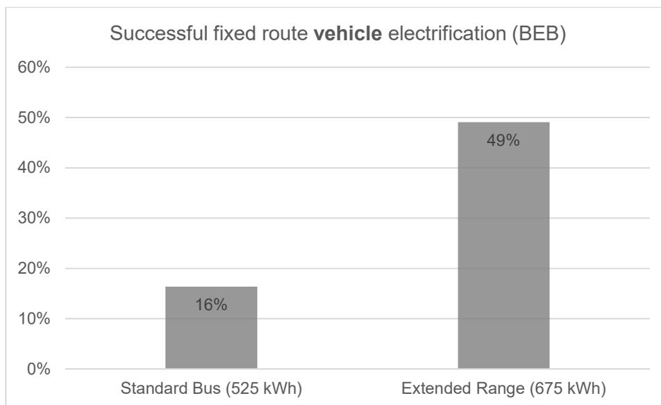
These results in Figure 11 indicate that without a larger battery size, only a small portion of vehicles (16%) can be successfully electrified. All blocks that use 30-ft buses were unsuccessful and no option for larger batteries currently exists. By modeling blocks operating with 40-ft buses with larger battery sizes, the success rate increased to 49%.
