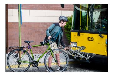
3. Place the bar over your front wheel (as close to the frame as possible).
